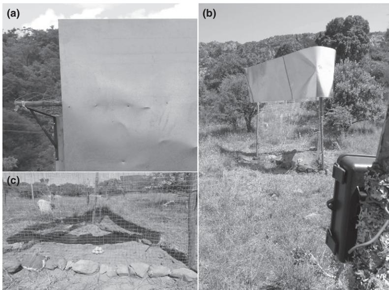
**Fig 2** Fence design with (a) the bracket positioned to hold the barrier away from the fence mesh, (b) the completed 3 m high enclosure with camera trap in foreground and (c) the position of bait in centre of enclosures
